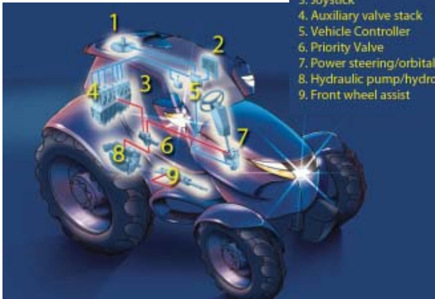
A typical hydraulic system for an agricultural tractor using propel with articulated steering.
